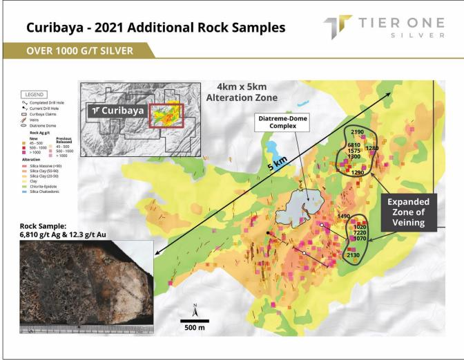
Figure 2: Illustrates the location of newly sampled high-grade silver-gold veins within the Curibaya alteration system as well as a newly identified zone of veining to the northeast of the defined chargeability anomaly.
