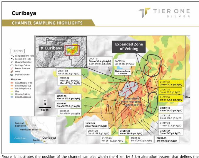
Figure 1: Illustrates the position of the channel samples within the 4 km by 5 km alteration system that defines the mineralized footprint on surface at the Curibaya project.
